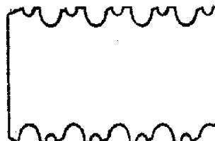
SSB SIGNAL, TONE INPUT BALANCED MOD DETUNED (L3)
